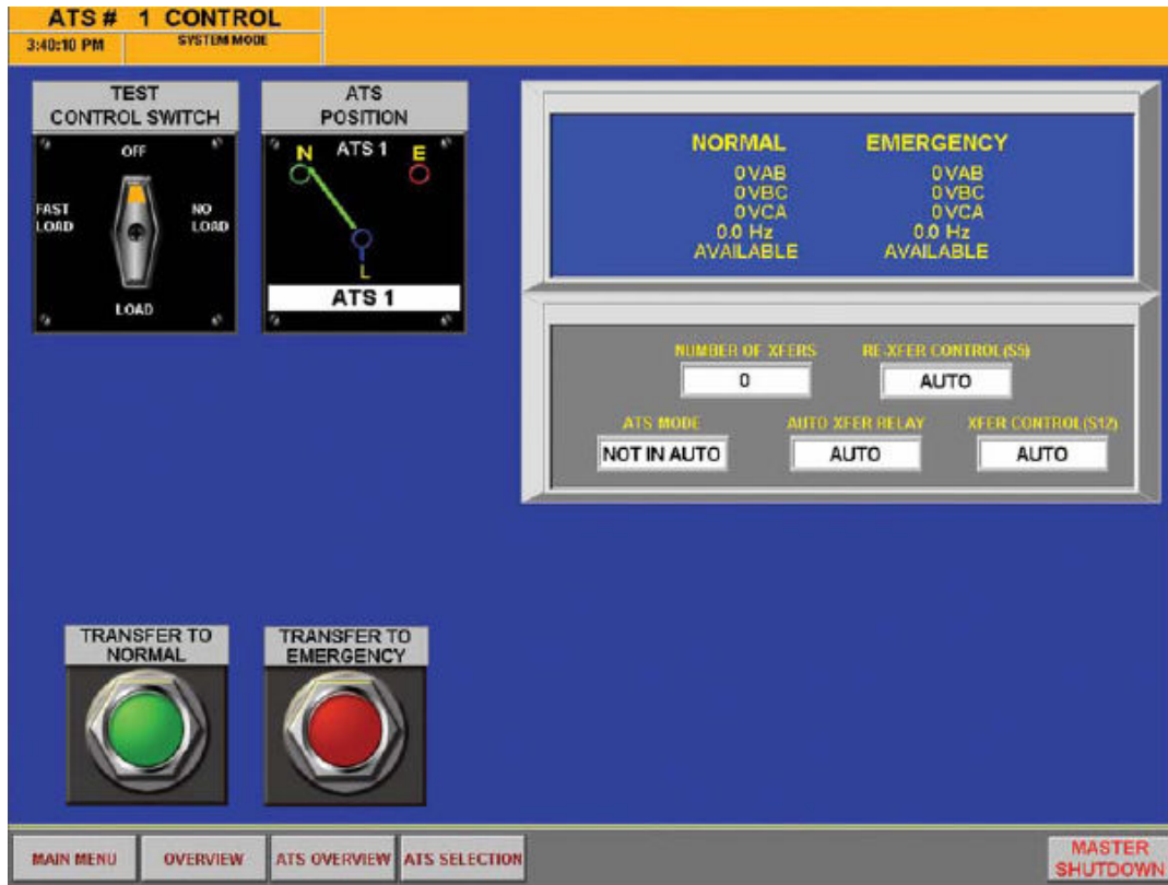
Figure 10 – ATS Remote Monitoring Software Screens
