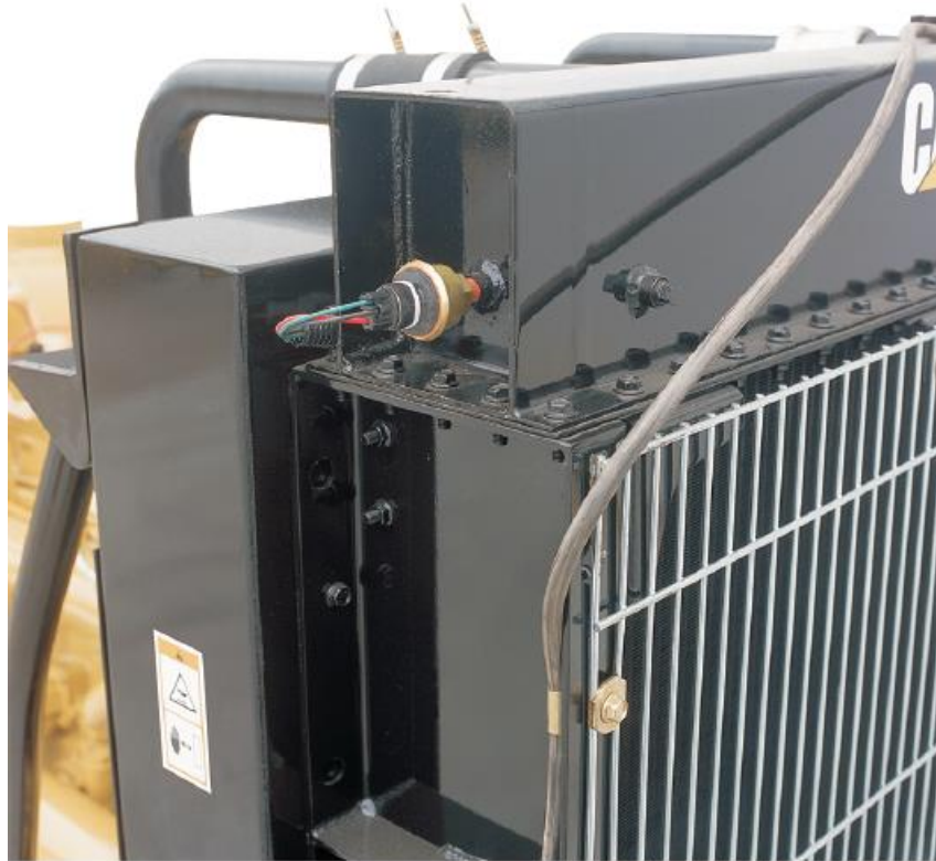
Figure 10: Coolant level sensor on a radiator for a Cat G3406 engine.
