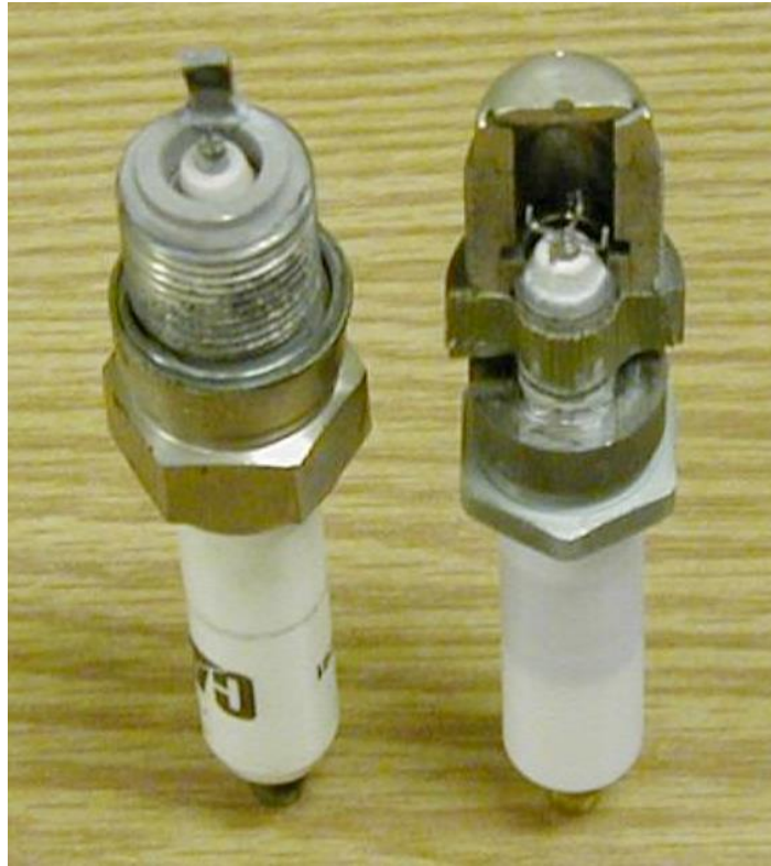
Figure 6: J-gap (left) versus prechamber (right) spark plugs.
