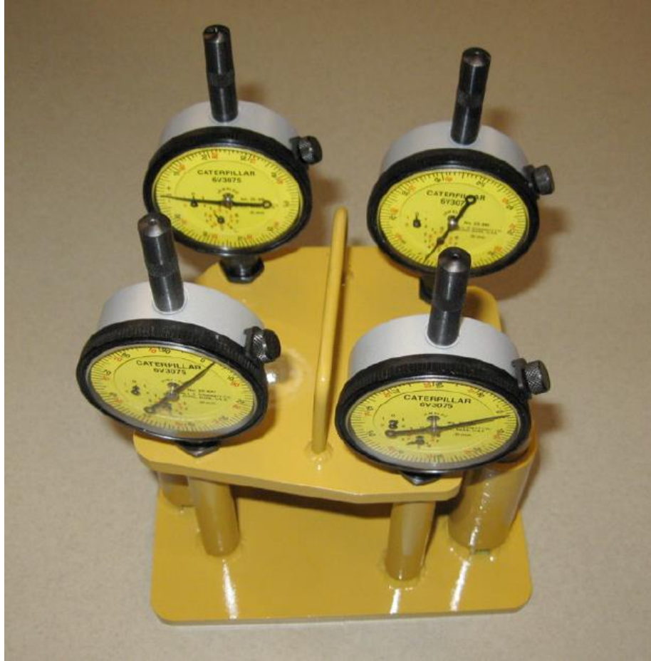
Figure 8: New valve recession measurement tool for Cat® G3500C/E engines.
